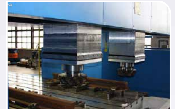
TUR RM 240 with two independent tool systems
