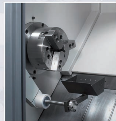
The retractable part catcher integrated with the front door outlet
